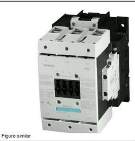
CONTACTOR, 55KW/400V/AC-3 AC(40...60HZ)/DC OPERATION UC 23...26V AUXIL. CONTACTS 2NO+2NC 3-POLE, SIZE S6 WITH BOX TERMINALS CONVENTIONAL OPERATING MECHAN. SCREW TERMINAL
